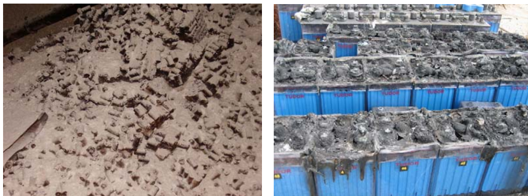
Figure 7.7. Partially Incinerated Dry and Liquid Batteries in Plastimed and Jiyeh (from left to right)
