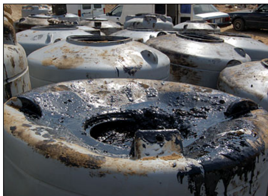
Figure 7.8. Large PVC containers used for storage of oil waste
